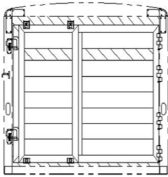
6'8" TALL, STANDARD LIVESTOCK SLIDER REAR OPENING - 90 1/2" X 76"
