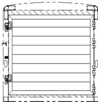
6'8" TALL, ENCLOSED SOLID GATE REAR OPENING - 90 1/2" X 76"
