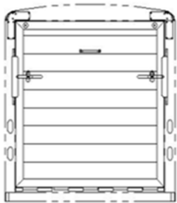
6'6" TALL, REAR RAMP REAR OPENING - 74 3/8" X 72 1/2"
